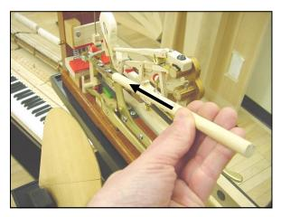
mentioned in Step 1, until the rod is in its correct position.
