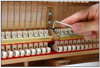
The distance between the rod and tabs can be established by means of a 3 mm Allen key at the three crossblock brackets (and with a 4 mm Allen key at the plate-nose bracket as shown in the photo below). The individual screws just need to be loosened and the brackets moved in the desired direction. Remember to tighten the screws immediately afterwards.
