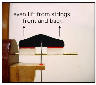
Step 4. Recheck damper lift—As a result of wire bending, the line of underlevers may need to be readjusted. Check for individual fast or slow dampers by operating the damper pedal, while observing the damper lift from bass to treble. Correct any fast or slow dampers by regulating the depth of individual damper wire into the underlever.
