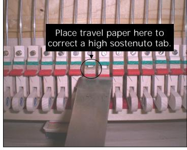
Step 3. Adjust the height of the sostenuto rod by using a sostenuto height gauge.
