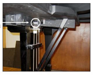
**Step 7. Adjust height of underlever tray**—Adjust the damper pedal rod so there is approximately 1/8" lost motion between the underlever tray and the line of underlevers.
