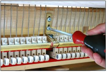
The height of the rod can be adjusted by loosening the screws that hold the three rod brackets to the crossblock and pushing the brackets up or down slightly.
