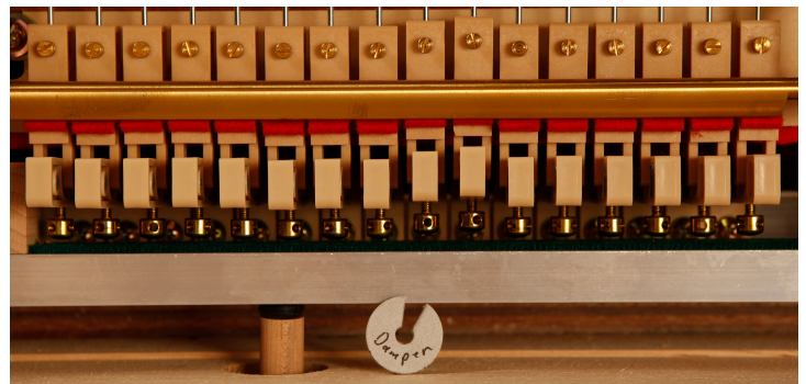
Sample levers are stepped, 2mm pitman shim is ready to be installed.
