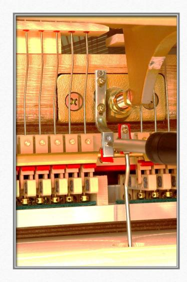
Remove pedal rods from damper and sostenuto pedals
