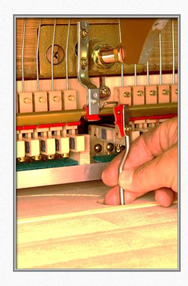
Loosen Sostenuto Rod Retaining Screws, turn clamp 90 degrees.
