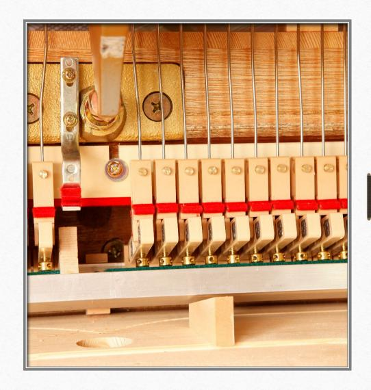
With action pulled forward, you can access the block screws.
