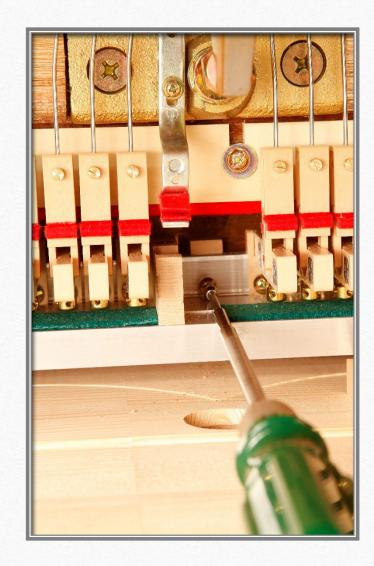
Lift dampers up, pull rail out.
